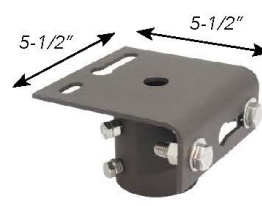
LF-AD-SF 2" slip fitter adaptor for LF flood lights with trunnion. Goes on 2" pipe and accepts a trunnion fixture.
